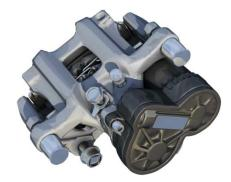
**Electric Parking Brake Caliper**
